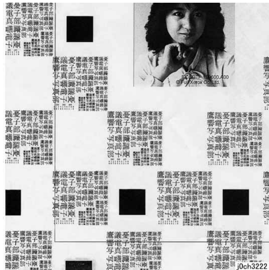
Figure 1 Toner Splattering Defect Sample (j0ch3222)
