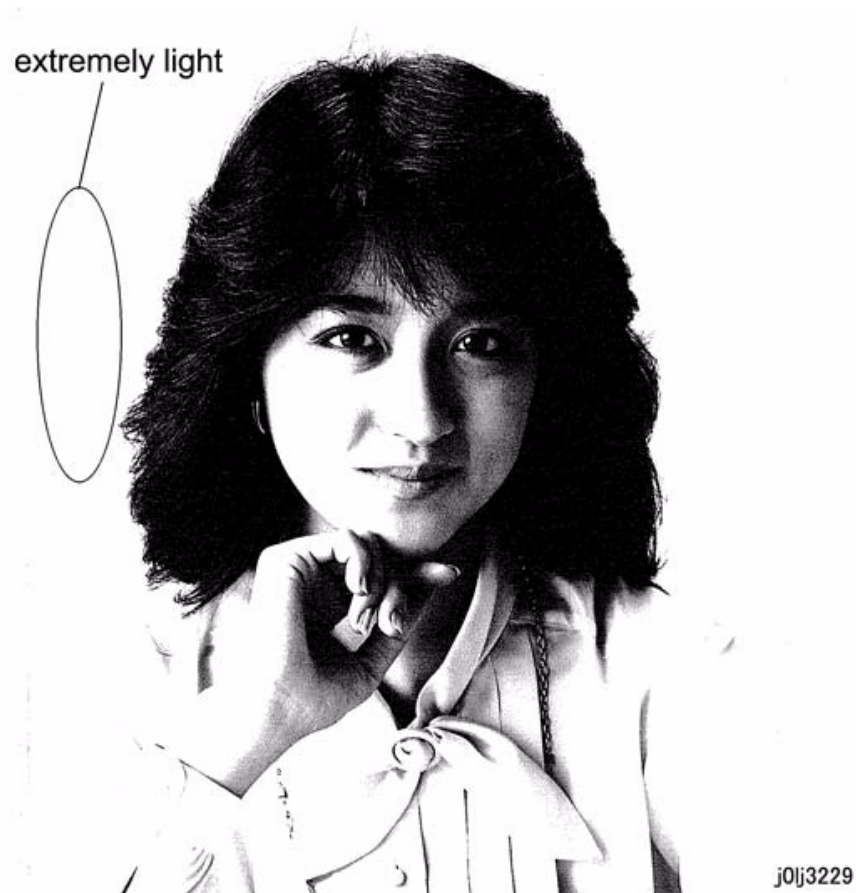
Figure 1 Light Background Due to Background Suppression in Copies of Documents With Frames Defect Sample (j0lj3229)
